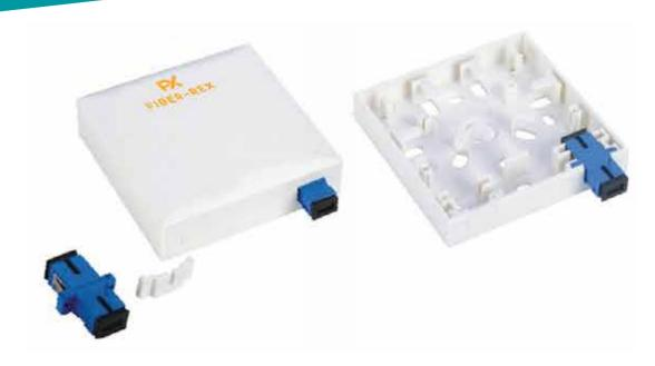
The compact fiber wall socket supplied by FIBER-REX is designed for residential and business applications and holds up to four fiber terminations. This wall box enables the installation of either a single Sirocco Blown Tube cables using up to a 2 fiber blown unit or two 2 fiber ruggedized cables to be spliced to 2 SC pigtails (PC or APC). The pigtails would which connect to adapters at the base of the unit.
